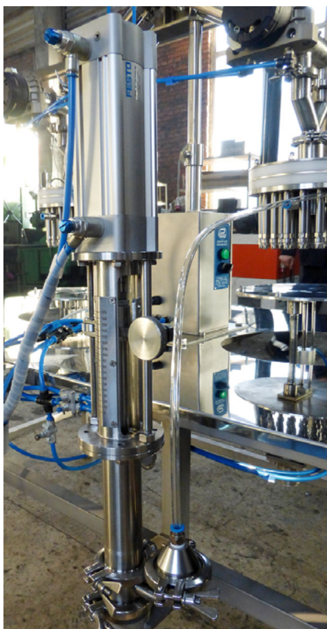
Dispenser for entering viscous products with a measuring scale
